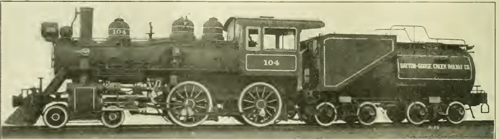
EIGHT-WHEEL TYPE 4-4-0 LOCOMOTIVE FOR THE DAYTON-GOOSE CREEK RAILWAY. BALDWIN LOCOMOTIVE WORKS, BUILDERS
